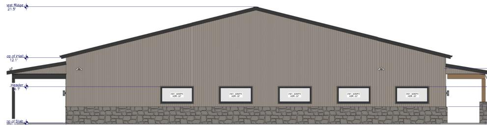
Exterior Elevation Left MATERIALS (EXCLUDES DOORS/WINDOWS & ROOF): R PANEL: 866 SF STONE PONY WALL: 212 SF (20%)
