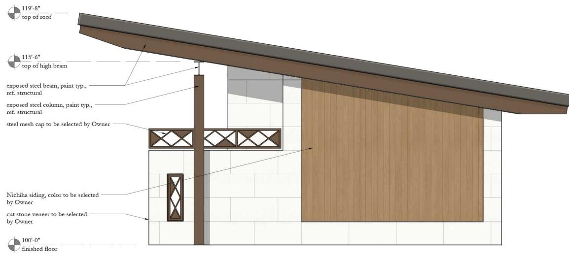
EAST ELEVATION - RESTROOM BUILDING ELEVATION SCALE: 1/4"=1'-0"
