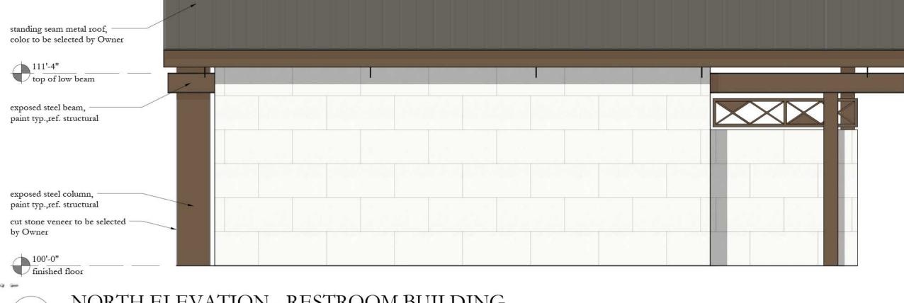
NORTH ELEVATION - RESTROOM BUILDING ELEVATION
