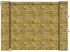
1: Rowlock Cap; 2: Running Bond; 3: 3/8" Tooled Joints (*Typical*); 2: Concrete Footing/Mow Strip.
