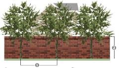
■: CANOPY TREES 20-FOOT ON CENTER; ②: MINIMUM SIX (6) FOOT MASONRY WALL;
