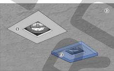
①: FLUSH LENS (I.E. FULLY RECESSED); ②: PROJECTING LENDS (I.E. NOT FULLY RECESSED); ③: CEILING
