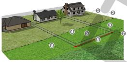
1: EXISTING RESIDENTIAL FENCE ON THE LEASING PROPERTY; 2: WROUGHT TRON OR BLACK TUBLAR STEEL FENCE; ③: MAXIMUM OF 45-FEET ALONG THE LEASE LINE OF THE TAKELINE; ④: REAR PROPERTY LINEJEGINNING OF THE TAKELINE; ④: 438.0 ELEVATION ZONE; ④: THE STRAIGHT-LINE CONNECTION BETWEEN THE TWO (2), 45-FOOT POINTS; ⑦: MAXIMUM OF 48-INCHES OR FOUR
