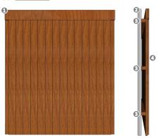
1: Top Rail; 2: Galvanized or Stainless-Steel Post (Recommended Minimum of 2.375"); **3**: Stinger Board (Recommended Minimum of 2" x 3"); **4**: Minimum ½" Wood Screen.
