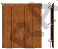
②: Top Rail; ②: Galvanized or Stainless-Steel Post (Recommended Minimum of 2.375"); ③: Stinger Board (Recommended Minimum of 2" x 3"); ③: Minimum ½" Wood Screen.
