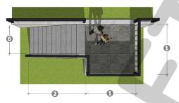
①: MINIMUM OF EIGHT (8) FOOT BY EIGHT (8) FOOT LANDING; ②: VARIABLE LENGTH STAIRCASE; ③: WROUGHT IRON, OR BLACK TUBLAR STEEL; ③: NATURAL STONE, BRICK, OR CONCRETE MATCHING THE RETAINING WALL; ③: VARIABLE HEIGHT BUT A MINIMUM OF THREE (3) FEET; ③: MAXIMUM OF SIX (6)
