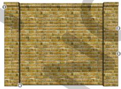
①: Rowlock Cap; ②: Running Bond; ③: 3/8" Tooled Joints (*Typical*); ②: Concrete Footing/Mow Strip.
