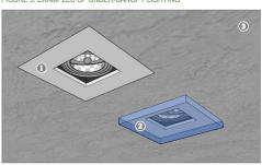
●: FLUSH LENS (*I.E. FULLY RECESSED*); ②: PROJECTING LENDS (*I.E. NOT FULLY RECESSED*); ③: CEILING
