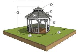
①: CUPOLA OR CLERESTORY; ②: 2:1 MINIMUM ROOF PITCH; ④: 1.5-FOOT MAXIMUM OVERHANG; ②: 18-FEET MAXIMUM HEIGHT WITH A CUPOLA OR CLERESTORY AND 15-FEET WITHOUT A CUPOLA OR CLERESTORY; ④: 12-FEET MAXIMUM; ③: ROOF CAN MATCH THE PRIMARY STRUCTURE OTHERWISE THE ROOF SHALL BE STANDING SEAM METAL.
