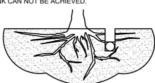
OPEN TRENCHING MAY BE USED IF EXPOSED TREE ROOTS DO NOT EXCEED 3" OR ROOTS CAN BE BENT BACK.
