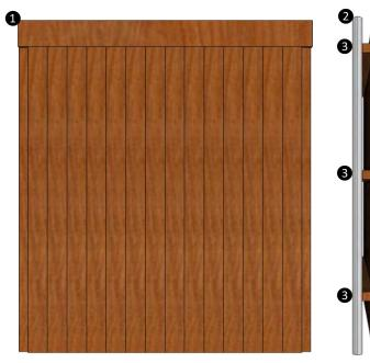
**1** Top Rail; **2** Galvanized or Stainless-Steel Post (*Recommended Minimum of*  $2\frac{3}{8}$ ); **3** Stinger Board (Recommended Minimum of 2" x 3"); **4** Minimum  $\frac{1}{2}$ " Wood Screen.
