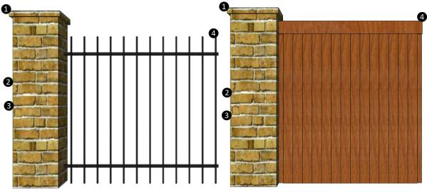
1 Rowlock Cap; 2 Running Bond; 3 3/8 Tooled Joints (*Typical*); 4 Wrought Iron or *Board-On-Board* Wood Fence.
