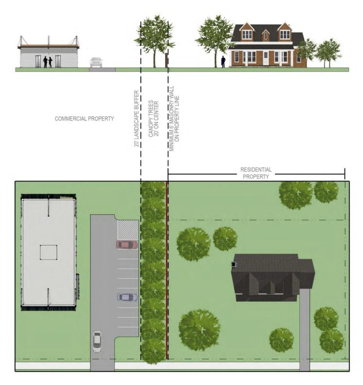
Figure 7: Masonry Fence with Canopy Trees in Perspective View
